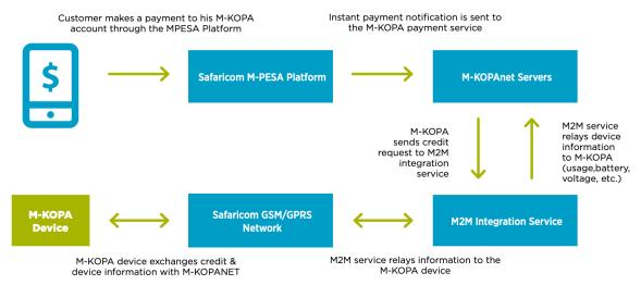
Figure 7: The M-KOPA machine-to-machine communication scheme is an example of how this technology could enable successful business models - Source: (GSMA, 2016)
